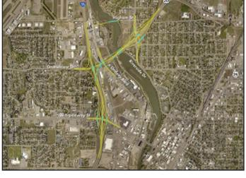
Alternative C includes adding lanes to separate the through-traffic from the local traffic between the I-15 Interchange Exit 118 (W Broadway St) and US-20 Interchange Exit 308 (City Center/Riverside Drive). Requires new retaining walls and bridges.
