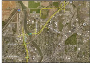
Alternative E (E.1 & E.2) relocates the existing I-15 Interchange Exit 119 to a new location closer to the airport. The alternative requires the addition of separated through lanes and frontage roads as well as the conversion of the existing US-20/Grandview roadway to a local street.
