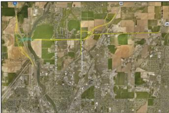
Alternative H realigns US-20 to the north and provides a connection to US-26 at E 49<sup>th</sup> N (Telford Rd). Existing US-20 between Johns Hole and E 49th N would require changes to convert it to a local street. I-15, Exits 118 and 119 would include safety and capacity improvements.
