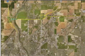
Alternative H realigns US-20 to the north and provides a connection to US-26 at E 49<sup>th</sup> N (Telford Rd). Existing US-20 between Johns Hole and E 49th N would require changes to convert it to a local street.
